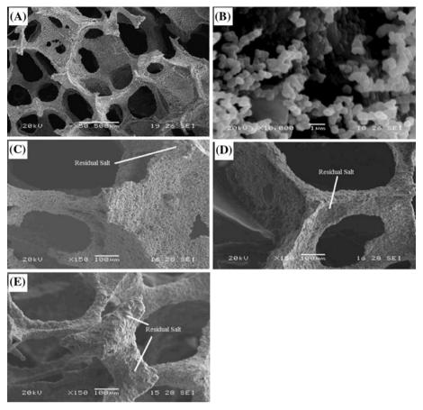
Nunzio et al. [8], as shown in Table 1. Figure 1 shows that whilst the porosity and the structure of the scaffolds have been maintained there is residual salt found on the surface of the scaffold (Fig. 1c-e), indicating that the scaffolds require a more rigorous washing process to solve this issue after the ion exchange process and that this should be addressed in the optimisation phase.
