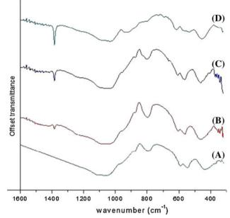
Fig. 11 FTIR analysis on scaffolds for the main concentrations of silver after the scaffolds were immersed in the salt bath for 30 min and after immersion in SBF for 15 days: **a** plain 45S5 Bioglass<sup>®</sup> scaffold, **b** low concentration  $Ag^+/45S5$  Bioglass<sup>®</sup> scaffold, **c** medium concentration  $Ag^+/45S5$  Bioglass<sup>®</sup> scaffold and **d** high concentration  $Ag^+/45S5$  Bioglass<sup>®</sup> scaffold
