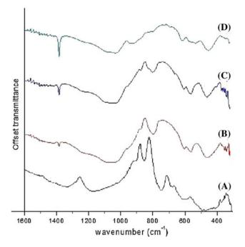
Fig. 8 FTIR analysis on scaffold surfaces for the main concentrations of silver after 60 min period of immersion in the salt bath: **a** plain 45S5 Bioglass<sup>®</sup> scaffold, **b** low concentration  $Ag^+/45S5$  Bioglass<sup>®</sup> scaffold and **d** high concentration  $Ag^+/45S5$  Bioglass<sup>®</sup> scaffold and **d** high concentration  $Ag^+/45S5$  Bioglass<sup>®</sup> scaffold
