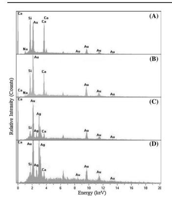
Fig. 2 EDX analysis on scaffolds for the preliminary concentrations of silver used in the ion exchange process: a plain 45S5 Bioglass<sup>®</sup>-derived scaffold, b preliminary low concentration  $Ag^+/45S5$  Bioglass<sup>®</sup> scaffold, c preliminary medium concentration  $Ag^+/45S5$  Bioglass<sup>®</sup> scaffold and d preliminary high concentration  $Ag^+/45S5$  Bioglass<sup>®</sup> scaffold
