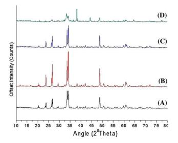
Fig. 3 XRD analysis of scaffolds for the preliminary concentrations of silver used in the ion exchange process: **a** plain 45S5 Bioglass<sup>®</sup> scaffold, **b** preliminary low concentration Ag<sup>+</sup>/45S5 Bioglass<sup>®</sup> scaffold, **c** preliminary medium concentration Ag<sup>+</sup>/45S5 Bioglass<sup>®</sup> scaffold and **d** preliminary high concentration Ag<sup>+</sup>/45S5 Bioglass<sup>®</sup> scaffold
