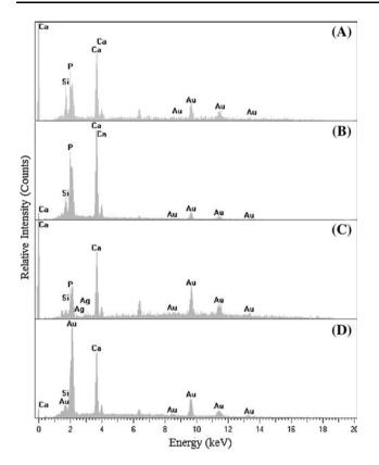
Fig. 10 EDX analysis of scaffold for the main concentrations of silver after immersion in salt bath for 15 min and after immersion in SBF for 15 days: **a** plain 45S5 Bioglass<sup>®</sup> scaffold, **b** low concentration  $Ag^+/45S5$  Bioglass<sup>®</sup> scaffold, **c** medium concentration  $Ag^+/45S5$  Bioglass<sup>®</sup> scaffold and **d** high concentration  $Ag^+/45S5$  Bioglass<sup>®</sup> scaffold
