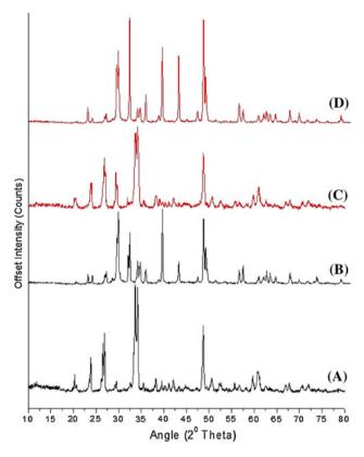
Fig. 7 XRD analysis on scaffold surfaces for the main concentrations of silver after an immersion period of 15 min in the salt bath: **a** plain 45S5 Bioglass<sup>®</sup> scaffold, **b** low concentration  $Ag^+/45S5$  Bioglass<sup>®</sup> scaffold and **d** high concentration  $Ag^+/45S5$  Bioglass<sup>®</sup> scaffold and **d** high concentration  $Ag^+/45S5$  Bioglass<sup>®</sup> scaffold
