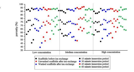
Fig. 5 Porosity study graph showing porosities for all three concentrations over all four immersion periods
