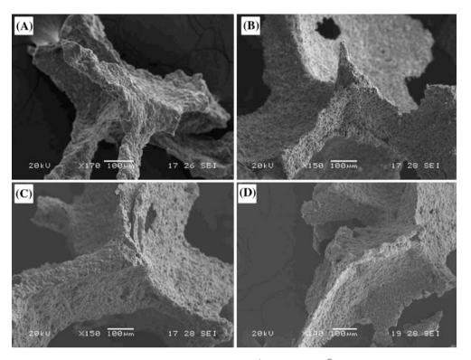
**Fig. 4** SEM images of scaffolds treated by ion exchange for 30 min at different concentrations: **a** plain 45S5 Bioglass<sup>®</sup> scaffold, **b** low concentration  $Ag^+/45S5$  Bioglass<sup>®</sup> scaffold, **c** medium concentration
