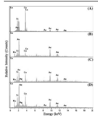
Fig. 6 EDX analysis on scaffold surfaces for the main concentrations of silver after immersion in the salt bath for 15 min: **a** plain 45S5 Bioglass<sup>®</sup> scaffold, **b** low concentration  $Ag^+/45S5$  Bioglass<sup>®</sup> scaffold, **c** medium concentration  $Ag^+/45S5$  Bioglass<sup>®</sup> scaffold and **d** high concentration  $Ag^+/45S5$  Bioglass<sup>®</sup> scaffold
